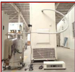
LN 2 /CO 2 backup system
